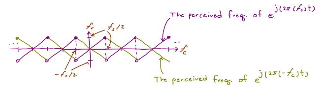
Observe that at every fc, for cos(217 fc+) its two complex- expo components always gives a pair of perceived freq., one positive and one negative (except when  $f_c$  is a multiple of  $f_{s/2}$ )
