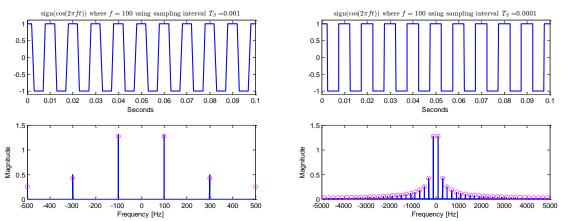
Our problem can be mitigated by reducing the sampling interval to  $T_s = 1/1e4$  instead of  $T_s = 1/1e3$  as shown by the plot on the right above.
