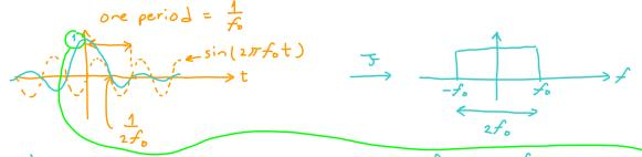
Then, we draw the sinc  $(2\pi f_0 t)$  using the zeroes of sin  $(2\pi f_0 t)$ We then see that the first zero occurs at  $\frac{1}{2f_0}$ . Therefore, in the freq. domain, the corresponding rectangular function has width =  $2f_0$ . So, its boundaries are  $\pm f_0$ . Conclusion: sinc  $(2\pi f_0 t)$  is band limited to  $B = f_0$ Note that the height of the rectangular function must be  $\frac{1}{2f_0}$  to make its area = 1.
